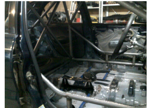
Looking into the car with completed roll cage & seat mounts
