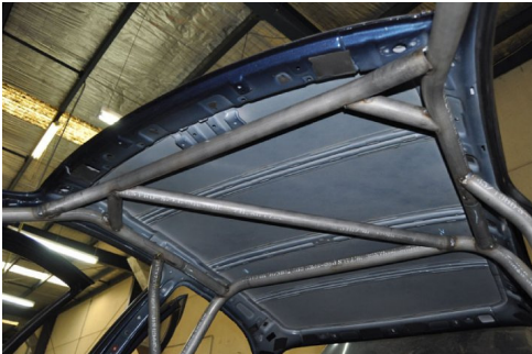
Progress is good on a roll cage, make it all feel real.
